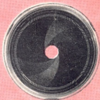
Smaller lens opening— larger number
